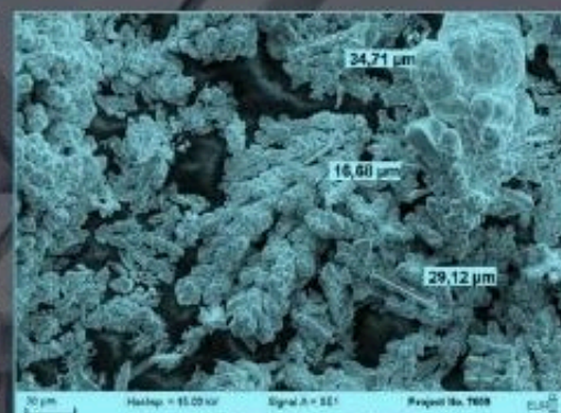
Dendritic structure 16 - 35 μm
